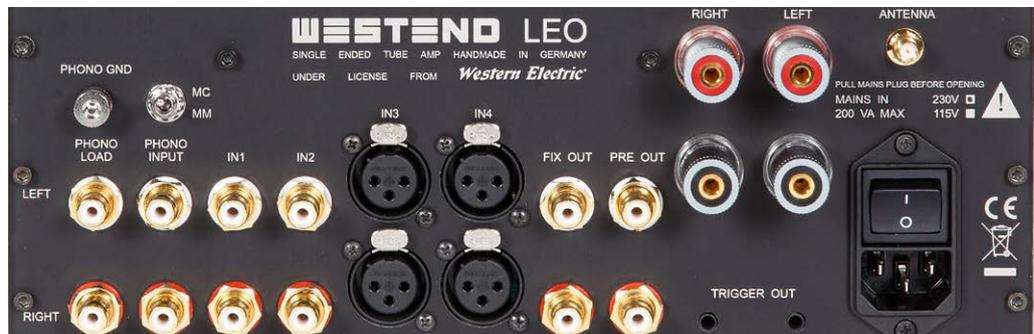
The connection panel offers sufficient possibilities to connect external sources. The XLR inputs are debalanced immediately; a Class A circuit is always unbalanced. Gold plated sockets – as befits this price range. The standby switch is located at the front and the mains switch at the rear.
