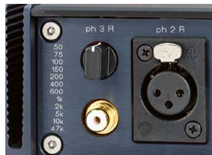
▲ The terminal impedance is finely adjustable, the variety of connections impressive.
