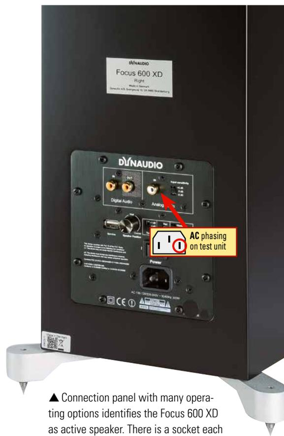
▲ Connection panel with many operating options identifies the Focus 600 XD as active speaker. There is a socket each for digital and analog signals.
