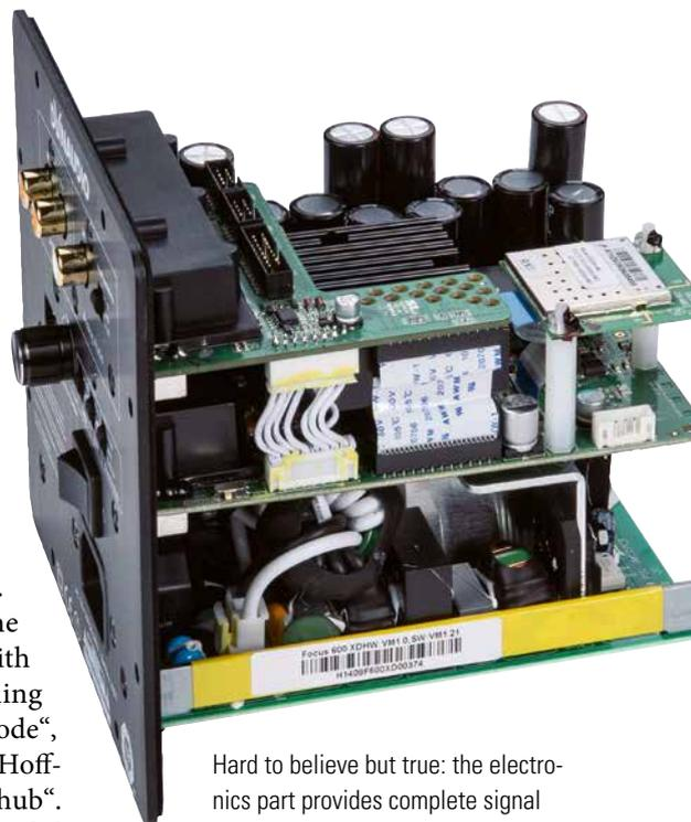
Hard to believe but true: the electronics part provides complete signal processing and four 150 Watt power amps in a very compact form.
