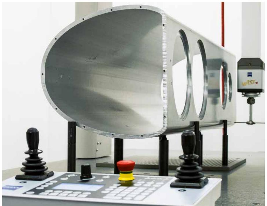
▲ The housing of the S3 is extruded under high pressure.
