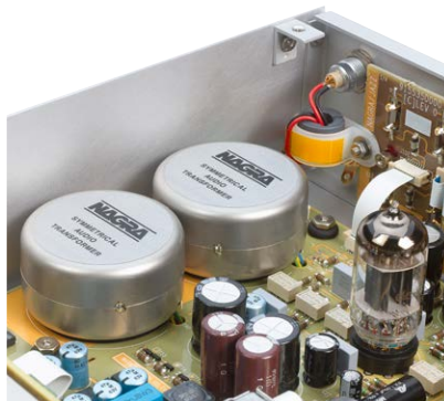
▲ The very high-value, encapsulated transformers are located directly in front of the symmetrical outputs.
