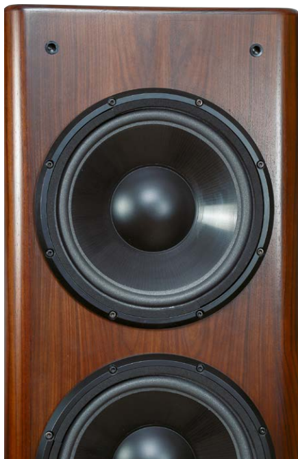
◀ A woofer with a new foam bead and stiffer dust cap than in the original.
