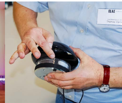
▲ The legendary 4Pi ribbon horn, with its 360-degree dispersion, is also built in Kiel.
