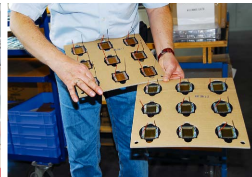
▲ Various jet tweeters with copper and aluminum foils after drying
