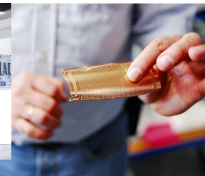
▲ The film of the jet tweeters is extremely thin and light.
