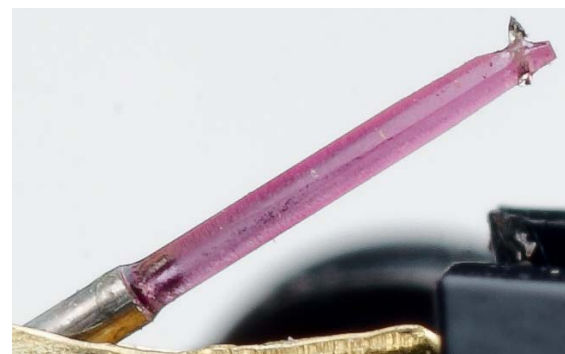
▲ The most expensive solution by far is the ruby cantilever – but it's also the more honest, and therefore preferable.
