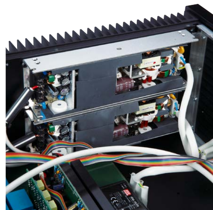
▲ Switching power supply units instead of thick transformers and electric batteries: the A 901 from its modern side
