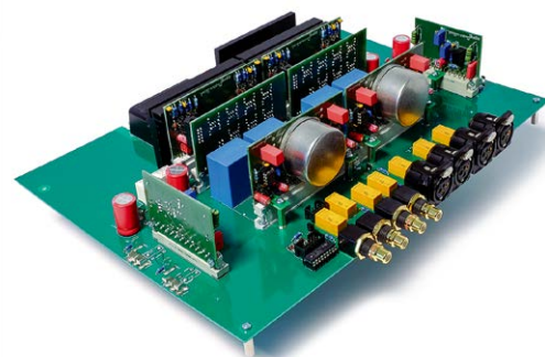
▲ Plug-in card technology ensures service-friendliness and updateability.
