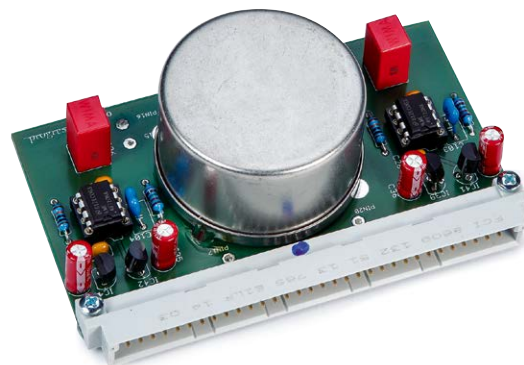
▲ The silver boxes are the input transformers built by Progressive Audio itself.
