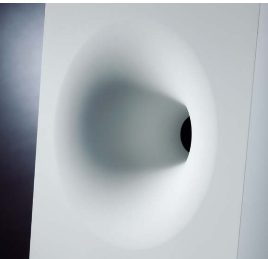
▲ The large fabric dome of the midrange driver lies in a horn opening measuring 40 centimeters at the outer edges.
