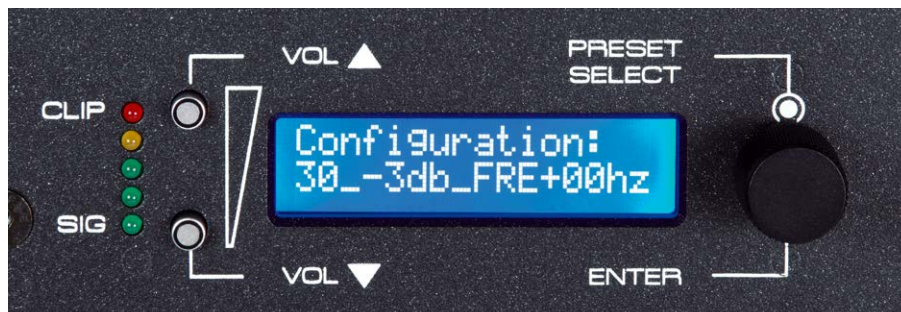
▲ One knob, two push buttons: With this minimum configuration you can easily jump through the countless preset memories of the Zero TA. The filter programming is better done on a PC.
