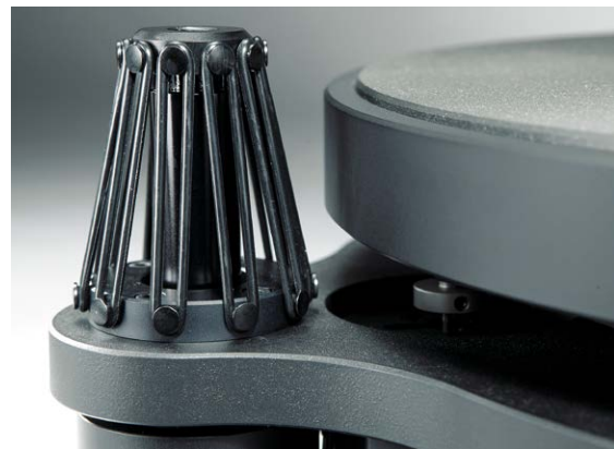
▲ The subchassis is suspended with ten rubber rings apiece from each of three domes. These rings last for a decade and are easily replaceable.
