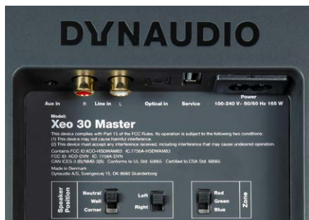
▲ The master speaker has four inputs (2 x analog, optical-digital and BT). Both speakers can be adjusted in the channel (left/right), pre-corrected for positioning close to walls and assigned to one of three room zones.
