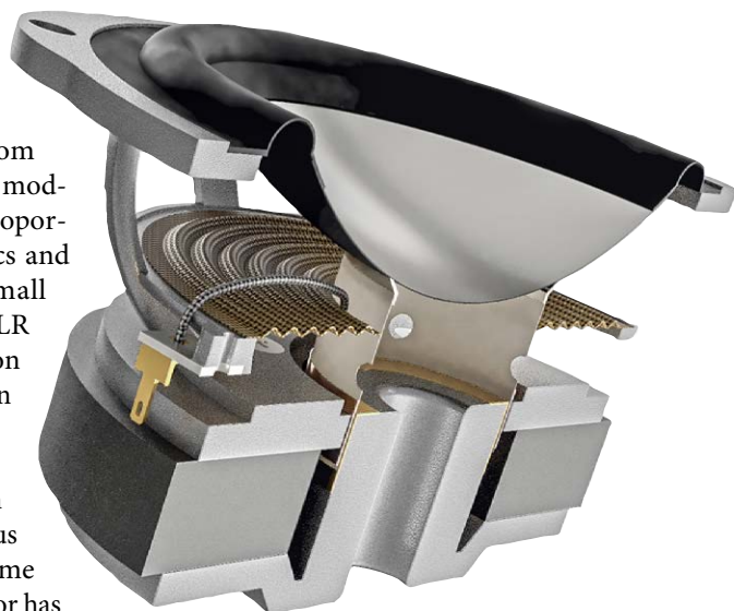
▲ Cross-section through one of the new Quadral drivers with "ALTIMA" membrane
