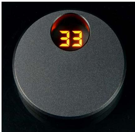
▲ The only control is a knob to select „Off“ and the two speeds, the values of which flash during start-up and only light up continuously after the selected speed has been reached.
