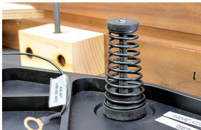
▲ The sub-chassis is suspended from three coil springs. In order to achieve an exactly piston-shaped swinging, these must be precisely adjusted.
