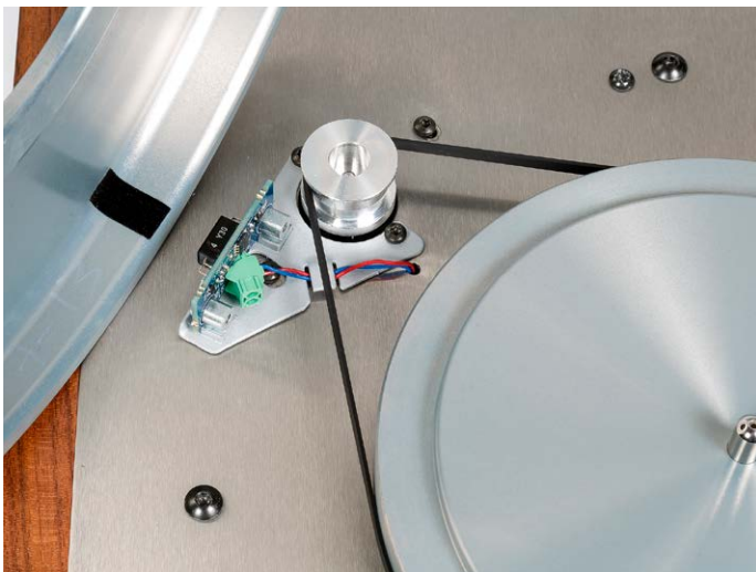
▲ A marking on the inside of the plate and an optical detector close to the engine ensure precise speeds. They were perfectly accurate!
