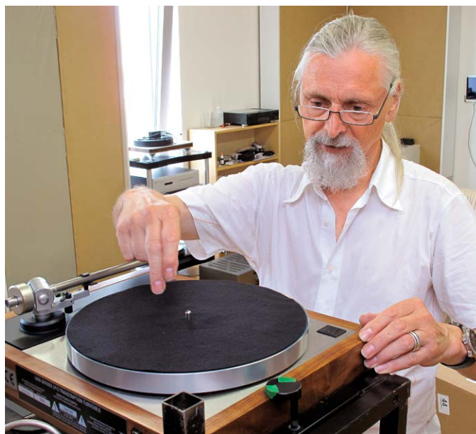
▲ The sub-chassis is suspended from three coil springs. In order to achieve an exactly piston-shaped swinging, these must be precisely adjusted.
