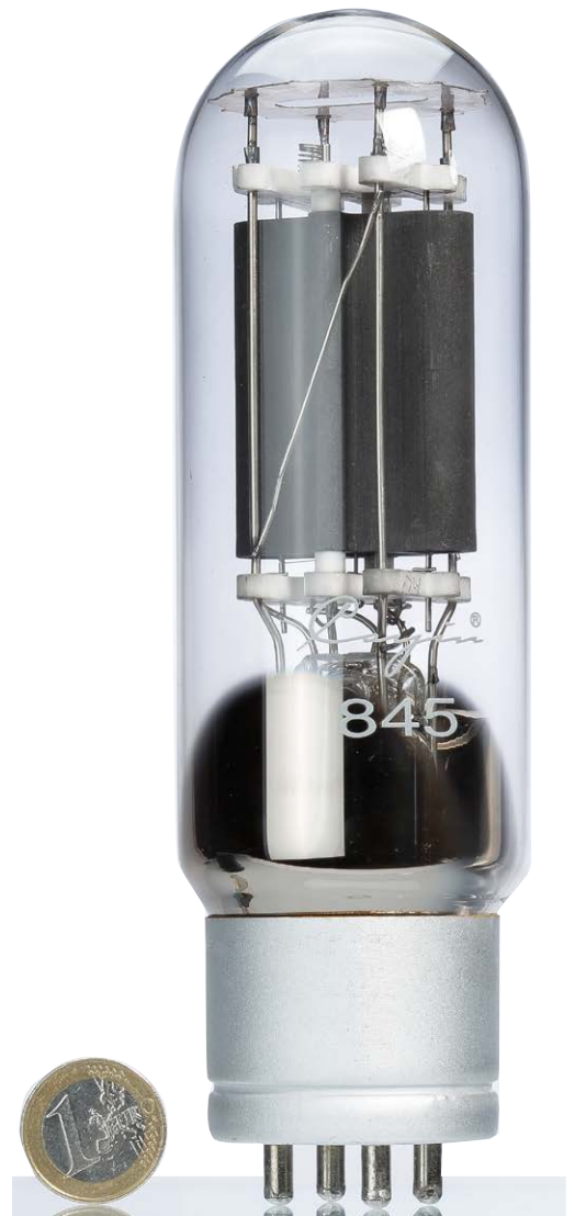
That’s a proper tube, isn’t it? The 845 is designed for single-ended class A operation. ▼
