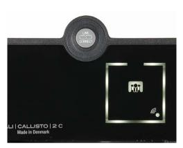
Use the "Link Connect" button on the back of the speakers to assign them to the left or right channel.
