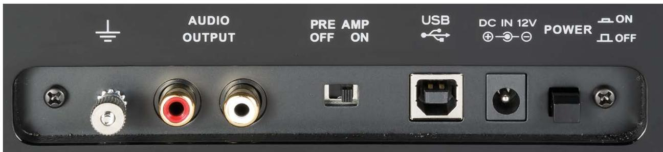
The signals are fed analogously from a pair of RCA sockets and digitally (16-bit/44.1 kilohertz) from a USB interface. When using an external one, the integrated Phono-Pre can be switched off.
