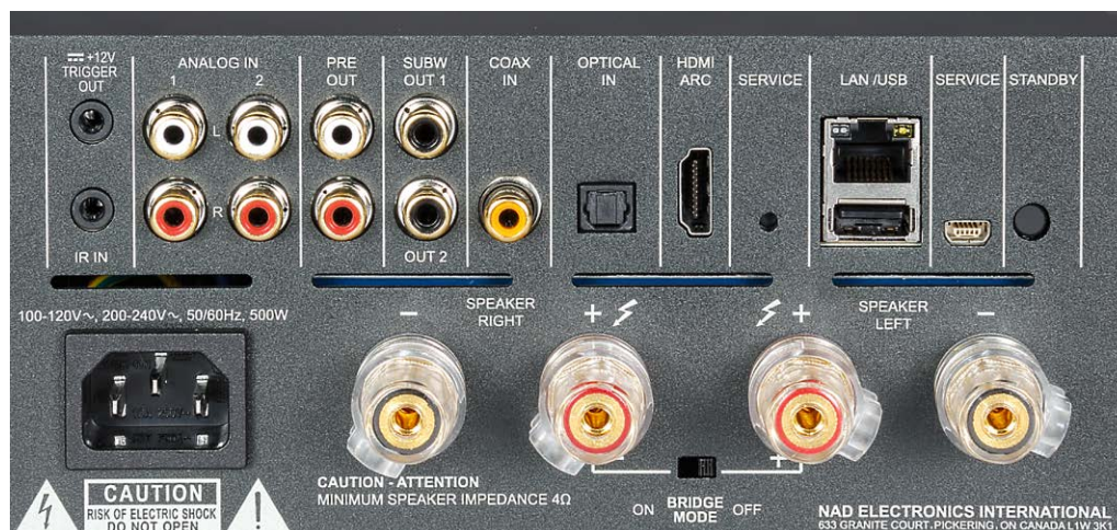
LAN/USB connector, analog and digital inputs, pre- and subwoofer outputs, bridge mode switch, solid speaker terminals and the convenient HDMI ARC input on the back.
