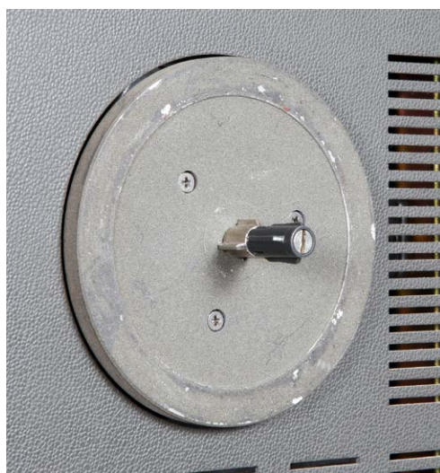
The Nextel coating of the tape plates has somewhat suffered; the clamping mechanism is plastic-coated.
