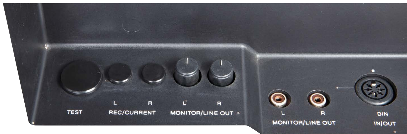
Rec/Current-control for adjusting the sensitivity to avoid level jumps between the pre/back-tape. The monitor controls can be used to adjust the output voltage.
