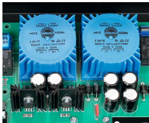
Two 25-watt transformers separately supply the digital circuits of the PLAYER I including drive and control as well as the D/A converter and output stage.
