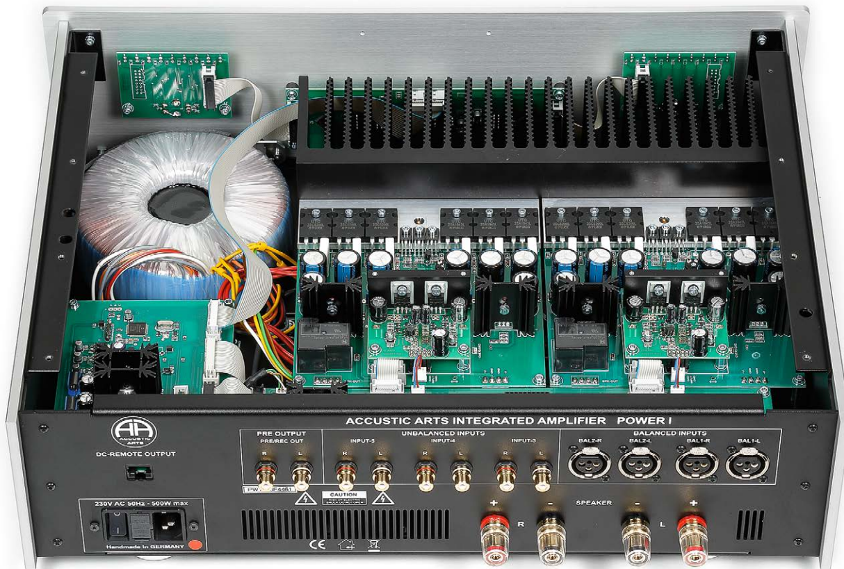
Six power transistors per channel are located on the heat sink. The 500-watt transformer is buffered by capacitors with 54,000 microfarads.
