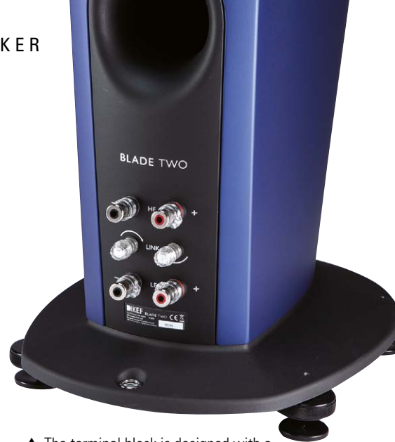
▲ The terminal block is designed with a special link mechanism to enable it to do without 'jumper bars' for single-wiring.
