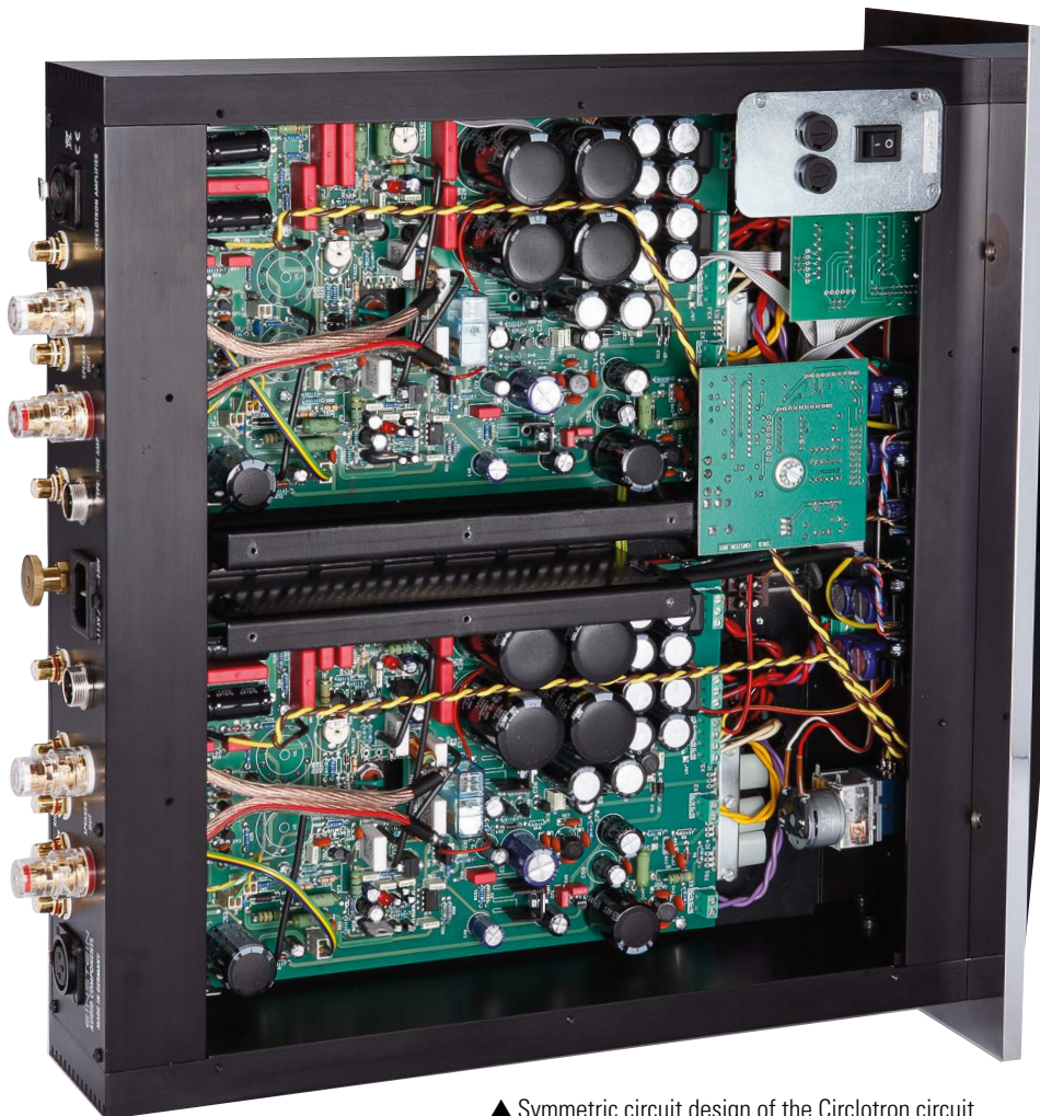
▲ Symmetric circuit design of the Circlotron circuit here implemented with transistors.
