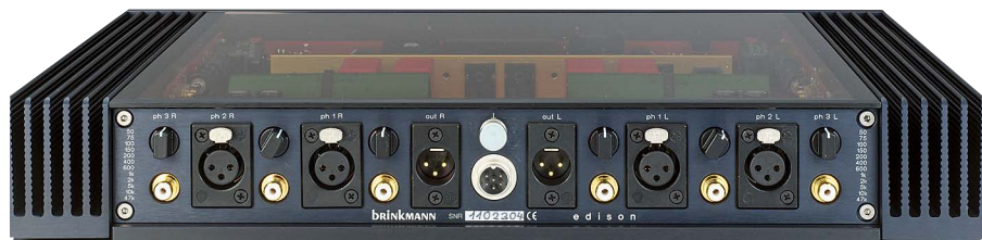
▲ The back shows single ended and balanced inputs and outputs and impedance adjustments
