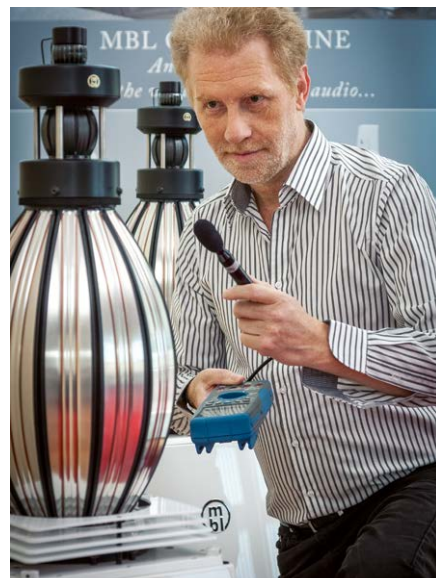
▲ The frequency response of the unique radial emitters has to drop slightly in the high treble
