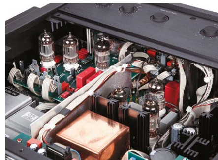
▲ Clever shielding and space for thermal management characterize the interior of the HP 700.
