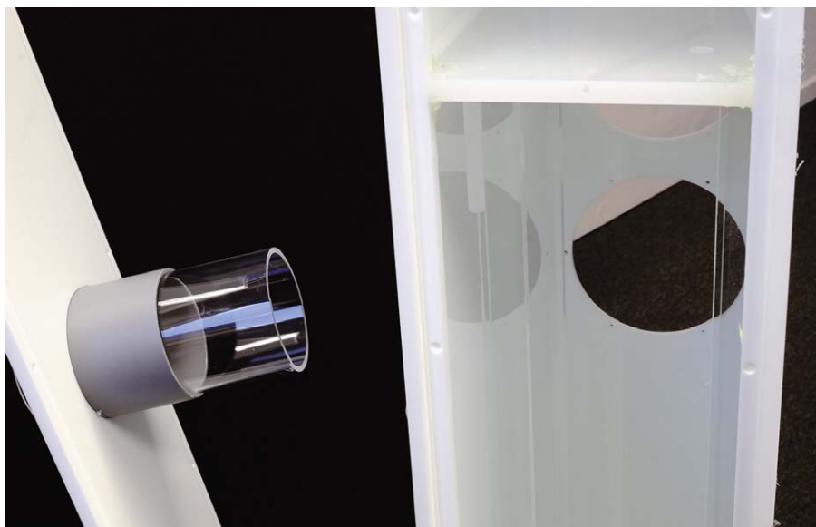
▲ The bass reflex tube is variable and can be adapted to any room to avoid bass droning – clever.
