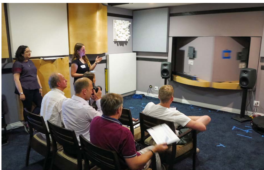
▲ Samsung's test room with its computer-controlled revolving wall enables blind comparisons of several systems. An acoustically transparent curtain (pictured) serves as a screen.
