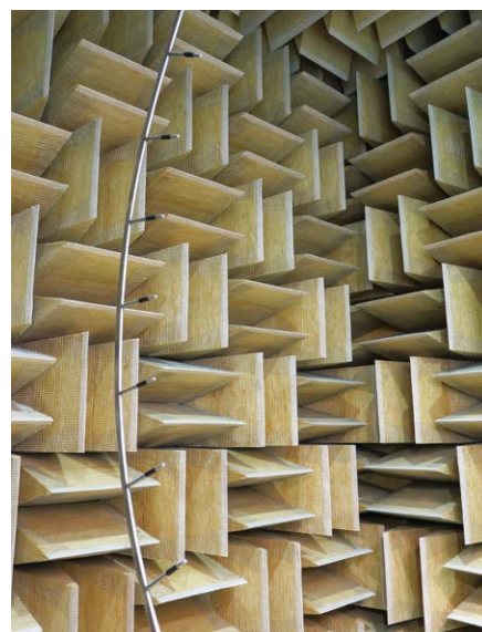
▲ With laser scanning (left), the Klippel system observes the displacement and distortion of the drivers at different frequencies and amplitudes. On the right is one of the two huge soundproof measuring rooms with its multi-point microphone system.
