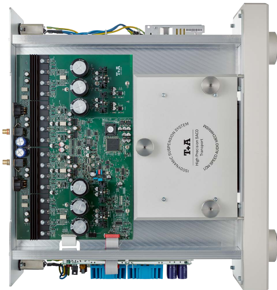
▲ The drive is decoupled and suspended at three points, while the MP 3000 antecedents remain visible in places.
