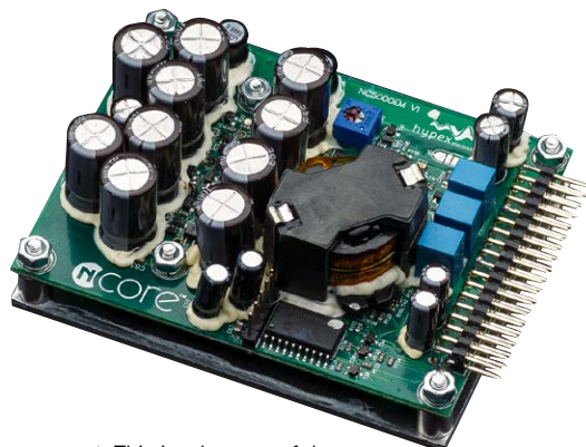
▲ This is what one of the four Marantz adapted mono power amplifier modules looks like.
