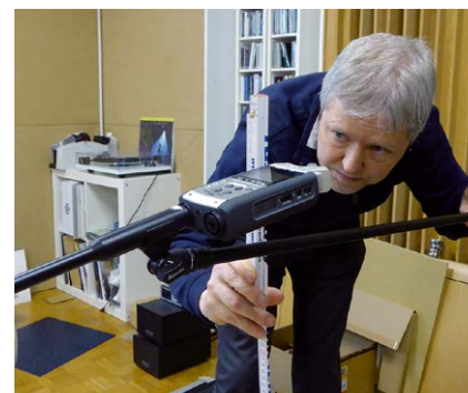
▲ Armin Krauss from Avantgarde Acoustic captured acoustic fingerprints of our large listening room from a total of five different positions.
