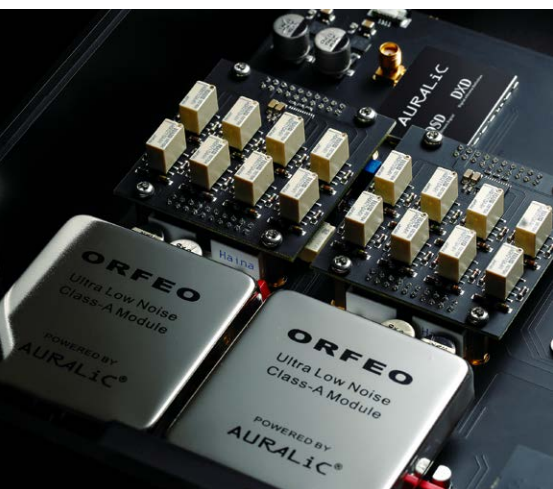
▲ The relays/resistor groups of the Vega G2's passive level control, and the Class A output stages, are accommodated on interchangeable boards.
