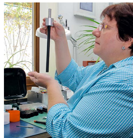
Giuseppina Schmeisser needs a sensitive touch to adjust the bearings of a tonearm. The arm must swing out at least 16 times to show the friction is low enough – and the bearing must be free of play.
