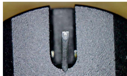
▲ The stylus had come loose from the cantilever of this high-end Mark Levinson MLC-1. Difficult, but in this case Schulte could help – price: €195.
