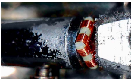
▲ Older EMTs often suffer from ailing, porous rubbers, Schulte observed. After the exchange, this one sounded like new, to the joy of its owner.
