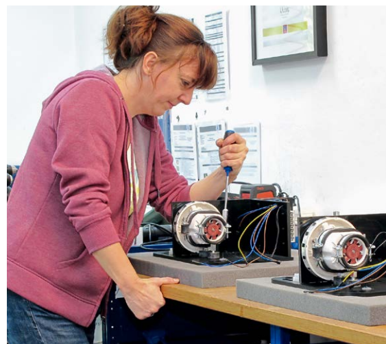
▲ Claudia Lux is working on the inside of a record cleaner, tightening the suction fan. When finished, the „Double Matrix Professional Sonic“, which cleans both sides of the record simultaneously, looks as classy and dignified as Clearaudio’s high-end turntables. Record cleaners are an important side of the business.
