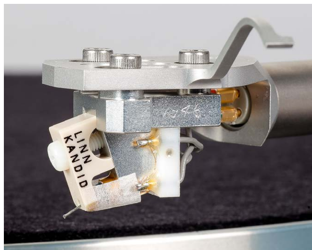
▲ The Kandid-MC is fixed with three screws, which increases the connection to the headshell and at the same time determines the overhang. Adjustment? Not required!
