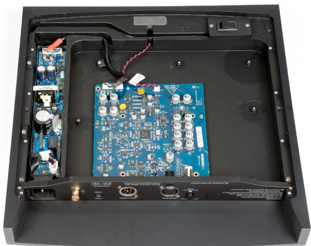
▲ In the Radikal unit, the supply voltages for the motor and preamplifier are generated with the utmost meticulousness. The switching power supply is located on the left.
