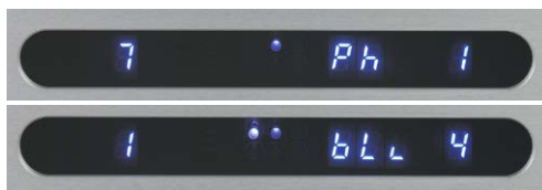
Two examples from the Amp menu: At the top, the headphone jack is activated; at the bottom, the balance is shifted to the left by the value „4“.
