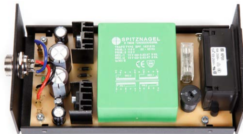
The external power supply is located in a metal enclosure and avoids interference fields inside the turntable. Its cable is one meter long.
