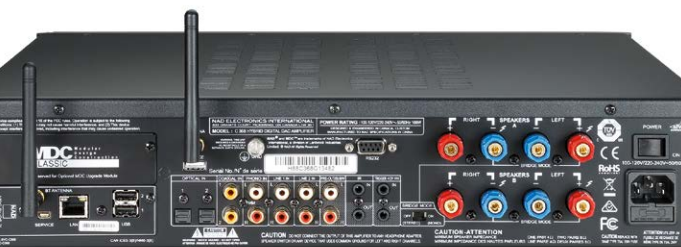
Bluetooth antennas as well as digital source channels represent the modern age. Phono (MM) is also on board. On the left you can see the optional streaming module with LAN and two USB slots.
