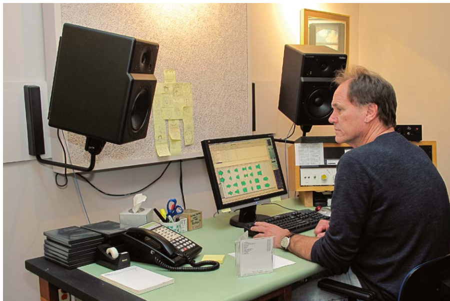
▲ For editing albums, a small set-up is sufficient in which the monitors are only used for recognizing the titles, for example at transitions
