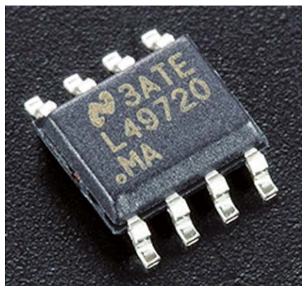
▲ High-precision operational amplifiers filter the signal currents for cinch and XLR completely separately.
