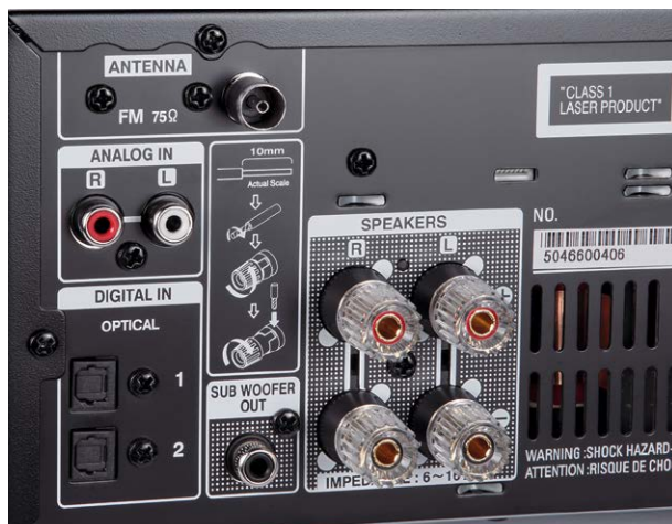
◀ The Denon has analog and digital connections for external players. You can also connect a subwoofer.
