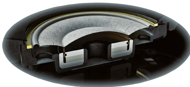
◀ The wafer-thin, but stable membrane from bacterial waste, the rubber surround (similar to a loudspeaker chassis) and the magnet drive, into which the voice coil is immersed, are clearly visible here
