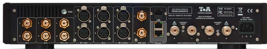
The amplifier provides three balanced and three cinch inputs, pre outs and connections for one pair of speakers. It can (optionally) be modified with a high-level input for turntable connection.
