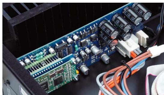
▲ With the optional USB circuit board, the Audia Flight becomes an external sound card.
