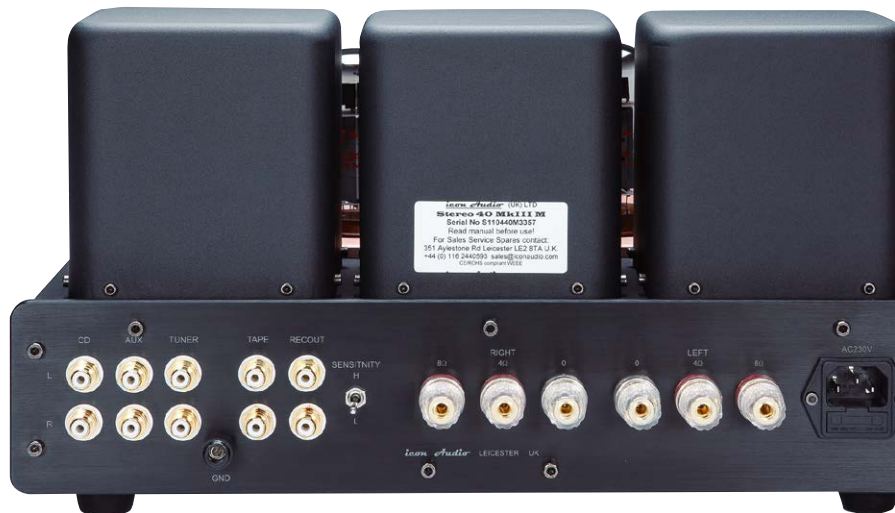
▲ Laudable: The input sensitivity can be switched between low and high
