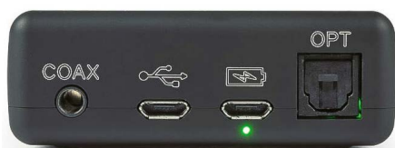
▲ Exclusively digital inputs: S/PDIF optical and as mini jack, USB micro, and a USB charge connection for the battery
