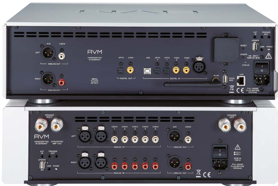
▲ In terms of connections, the AVM system will leave little to be desired. Amp and player share the work load. An external preamp would only be needed for a record player.
