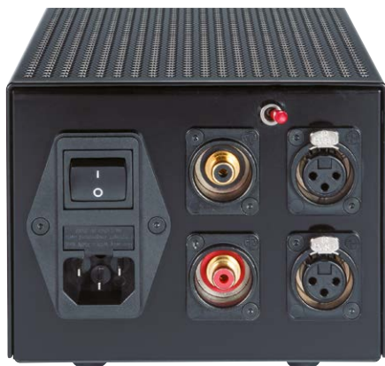
▲ The toggle on top controls a relay to switch between the cinch and XLR inputs.
