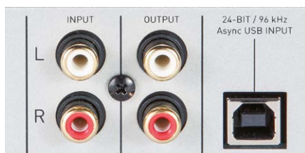
Analog input and USB port. You can connect for instance a recorder to the fixed-level output. ▲
