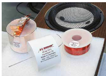
▲ Marten's crossovers use selected high-quality components, including Mundorf capacitors and condensers from Danish company Jensen.
