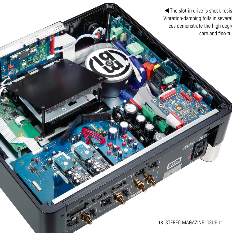
▲ Questions about the concept of the N31? The complexity of the boards arranged next to each other for the analog and digital inputs and outputs demonstrate serious intent as a DAC as well as a disc-player.
