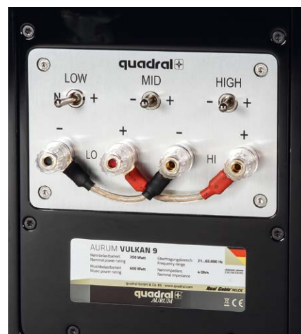
▲ Room correction: the bass can be raised, mids and trebles can be raised or lowered.
