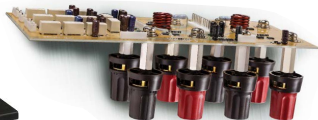
▲ The contact between the output board and the generously dimensioned connection terminals is established via metal rails.
