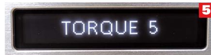
▲ The OLED display of the supply unit, which can be dimmed, turned off and switched, informs about the deviation from the setpoint speed 1 , shows the selected speed 2 and allows specific settings down to the second decimal place 3 . It also allows control of the engine torque. At „Torque 1“ it is weak 4 , at „5“ it is at maximum 5 .
