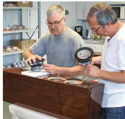
▲ Marten uses high-quality chassis with stiff, light ceramic membrane by the German specialist Accuton. Here, two deep/mid-rangers are being placed in a Miles5 (12,000 €/pair).
