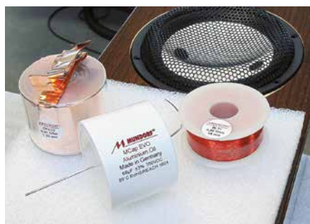
▲ Marten's crossovers use selected high-quality components, including Mundorf capacitors and condensers from Danish company Jensen.
