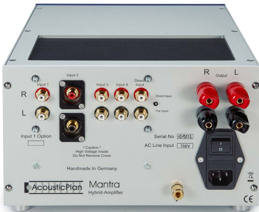
▲ While Input 1 can optionally be transformed into a phono input, Input 2 can be balanced if desired – for which it is already mechanically prepared.
