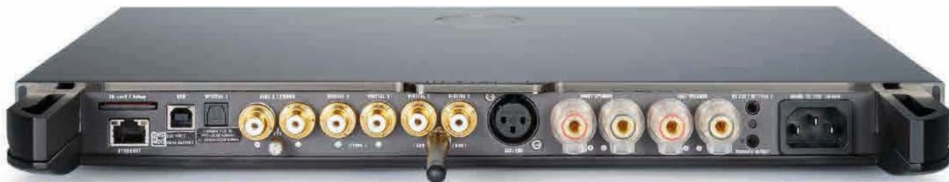
▲ The sockets and interfaces on the rear of the amplifier are tightly packed. There is a Wlan antenna as well as a ground terminal for the input, that handles phono signals unless otherwise configured. At the top left is the slot for the individually programmed SD card.
